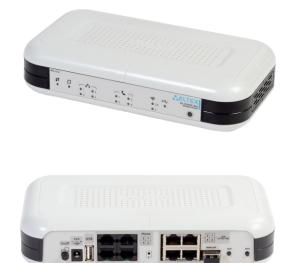
**RG-1504GF-Wac** is a high performance VoIP gateway with a built-in router. The device supports various services: VoIP, IPTV, high-speed Internet, dual-band Wi-Fi that can operate simultaneously in 2.4 GHz and 5 GHz.
