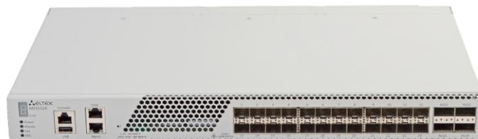
**MES5324** switches are high performance devices with 10GBASE-R and 40GBASE-SR4/LR4 interfaces that can be used as aggregation switches in carrier networks and as Top-of-Rack or End-of-Row switches for data centers.
